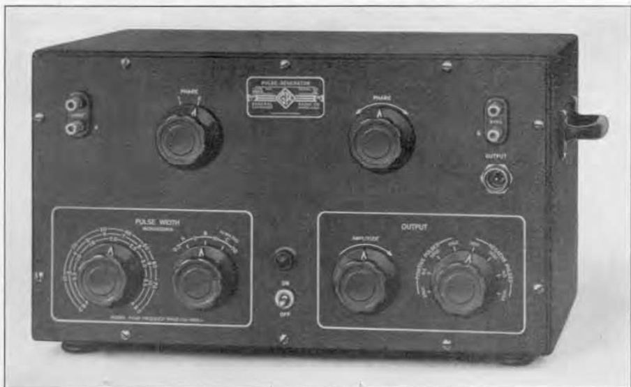
FIGURE 1. View of the TYPE 369-A Pulse Generator, showing panel and controls.
